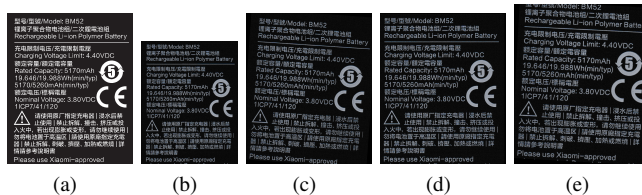
Fig. 4: A set of LBCSP images: (a) template image; (b) scale, the scale range is within [0.5, 1.5] times of the template image; (c) rotation, the rotation range is within [-5°, 5°]; (d) shift, the shift range is within [0.5, 3] pixels; (e) affine, images contain 2 or 3 of the above stated changes.
